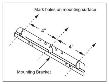
Figure 2. **Mark Holes using Power Center Mounting Bracket**
