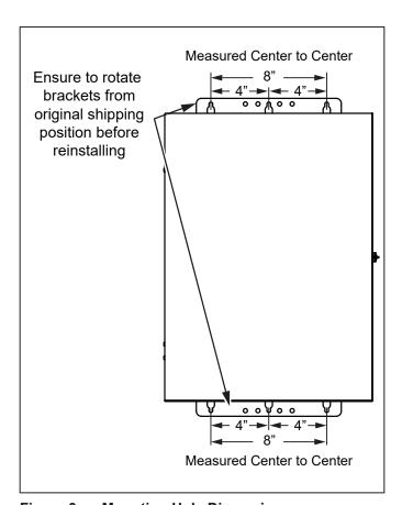
Figure 3. **Mounting Hole Dimensions**
