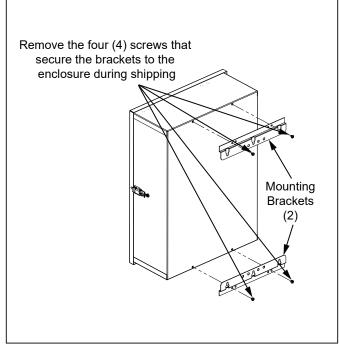
Figure 1. Enclosure Installation
